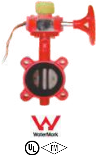
Lugged Butterfly Valve DI (300 PSI) Gear Operated with Tamper Switch-UL/FM Approved
